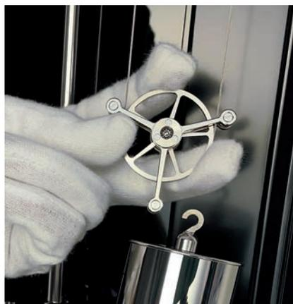
Wind the clock with the crank one turn counter clockwise. Deflect the pendulum until a “tick”, caused by the drop of the escapement wheel tooth on the pallet, is audible. Watch the pendulum scale and note the angular minutes, indicated by the tip of the pendulum, exactly in the moment where the “tick” occurs. Now deflect the pendulum to the other side and again note the angular minutes when the “tick” is audible. It is ideal, when the angular minutes are equal on both sides.
