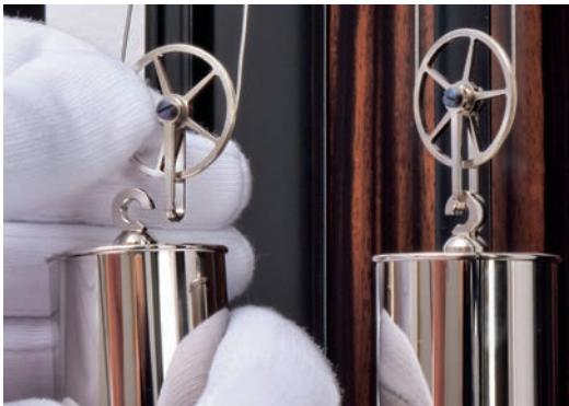
Then hang the weights in the bow of the rope pulleys without bending the cables.
