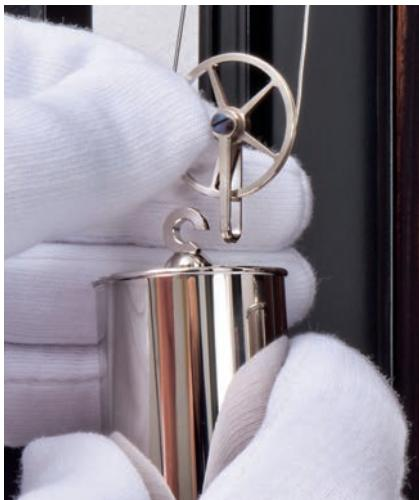
Then hang the weight in the rope pulley without bending the cat-gut.
